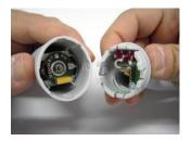
2. Push the motor and chuck mechanism out of the motor jacket as shown below
